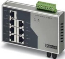
Ethernet Switch, 7 TP RJ45 ports, 1 FO port, 100 Mbps full duplex in ST-D format, automatic detection of data transmission speed of 10 or 100 Mbps (RJ45), autocrossing function
